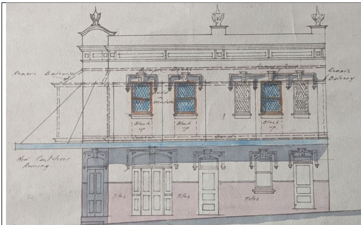
This elevation plan shows the Devonshire Street façade of the Clarendon Hotel with an outline of the original balcony to be demolished and a new awning. The 'Proposed alterations to Clarendon Hotel...for M Halpin Esq.' by architect Francis P Ryan, were approved October 1924 (City of Sydney Archives, A-00556071, https://archives.cityofsydney.nsw.gov.au/nodes/view/1424647 )
